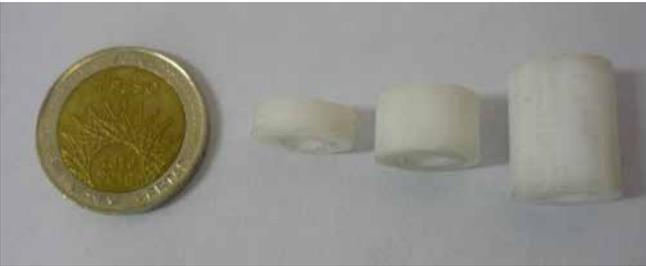
Fig. 14: Teflon slabs of thicknesses  $d = 4$  mm,  $d = 8$  mm and  $d = 16$  mm.
