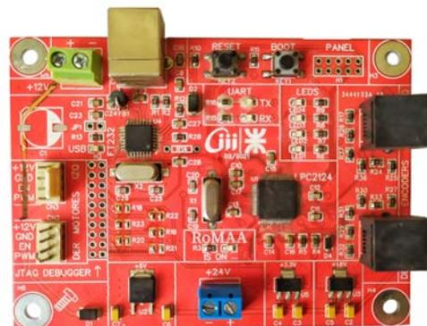
Fig. 3: Old version of the differential-drive robot controller based on a  $\mu C$  without ROS 2 support.
