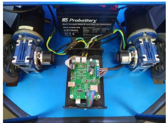
Fig. 8: New differential-drive robot controller mounted on RoMAA-II robot.
